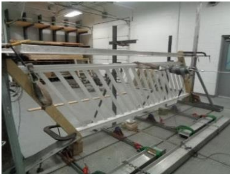
Photo No. 6 Concentrated Load at Midspan of Top Rail - Trademark
