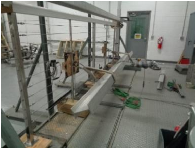
Photo No. 3 Infill Loading at Center of Both Intermediate Balusters
