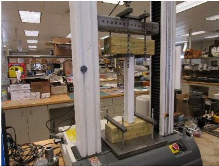
Photo No. 1 Assembly Fastener Test Setup
