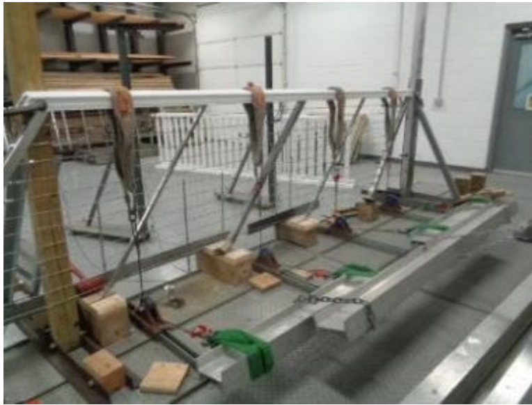
Photo No. 5 Vertical Uniform Load on Top Rail
