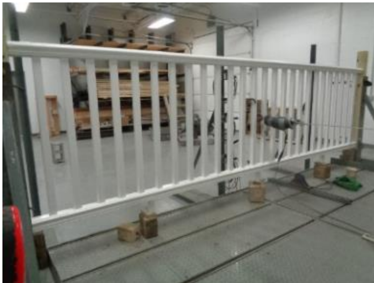
Photo No. 2 Infill Loading at Center of Two Balusters
