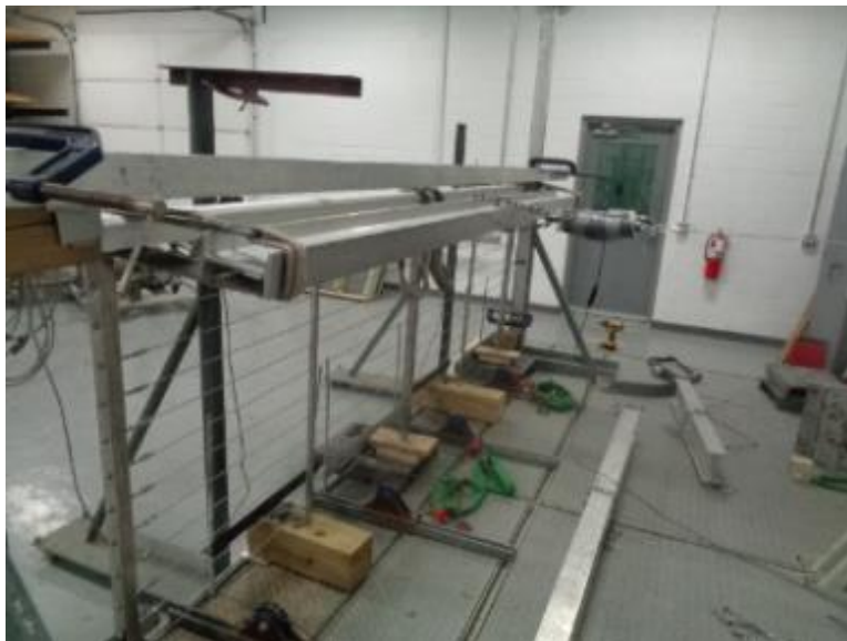
Photo No. 8 Concentrated Load at Both Ends of Top Rail (Brackets)
